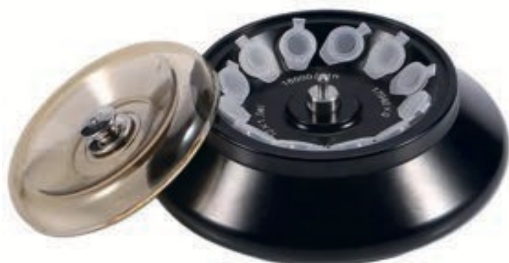
Rotor angulaire 12×1.5/2ml, 16000 rpm
